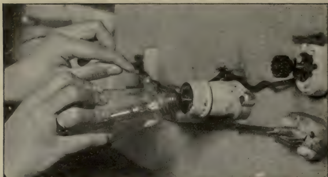
FIG. 129. How the lamp and wire are held to ground the circuit.
